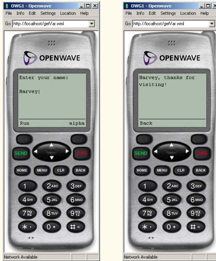
Fig. 23.13 Setting and displaying a variable using WMLScript (part 2 of 2). (Image of UP.SDK courtesy Openwave Systems Inc. Openwave, the Openwave logo, and UP.SDK are trademarks of Openwave Systems Inc. All rights reserved.)
