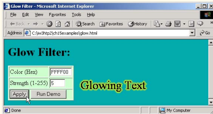
Fig. 15.7 Applying changes to the glow filter (part 3 of 3).
