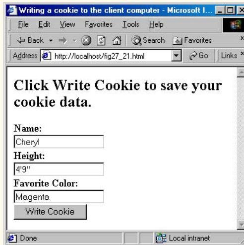
Fig. 27.21 XHTML document to read in cookie data from the user (part 2 of 2).
