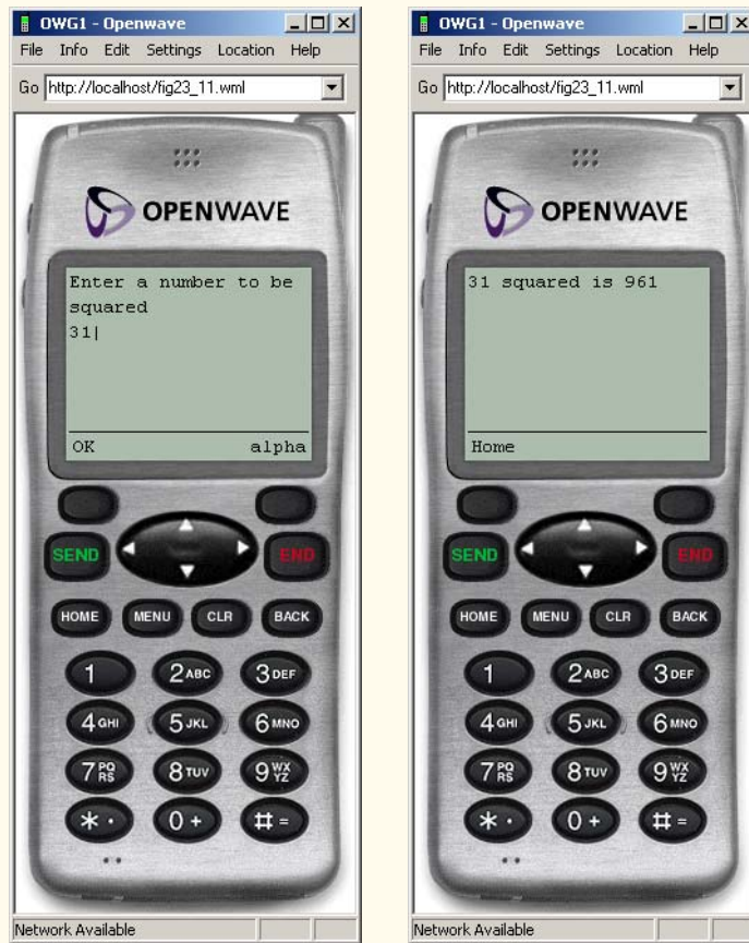
Fig. 23.11 Squaring a number by using programmer-defined functions (part 2 of 2). (Image of UP.SDK courtesy Openwave Systems Inc. Openwave, the Openwave logo, and UP.SDK are trademarks of Openwave Systems Inc. All rights reserved.)
